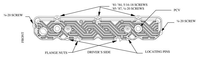
On the driver's side of your cover are 2 locating pins which engage holes on the cylinder head and help keep the gasket in position. Also note the 2 flanged nuts that clamp the driver's side of the cover to the head. Our cover makes use of both of these features.
